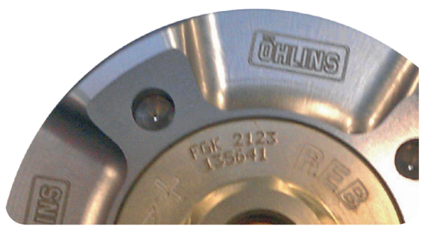
The part number is on the top cap.
